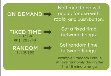
6. Factory timing is set to Random Max 30, which means that the AirScare will go off at least once every 30 minutes.
