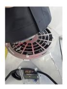
3. Attach the duct with the fabric to the base by lining up the four metal tabs with the corresponding slots. Twist the duct clockwise to lock it in place.
