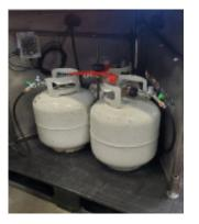
6. Tighten the black knob on the threaded rod until the hold down clamps firmly secure the propane tanks. Then open the propane valves and press each green safety valve.
