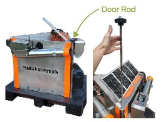
2. Once the door rod has been removed gently lift the cannon barrel and swing the door open.
