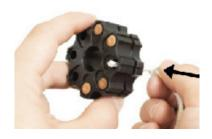
3. Poke the safety pin through the cylinder at a slight angle to push out the spent blanks.
