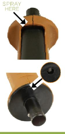
1. Pull the trigger in and spray a silicone based lubricant into the hollow area. Pull the trigger again several times in order to spread the lubricant.
