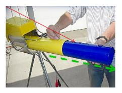
5. Attach Rotator Cup (#92306) to the end of the barrel.
