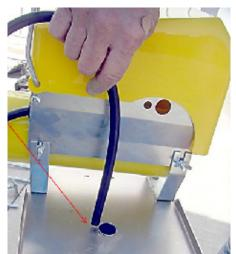
3. Reattach Regulator to hose using supplied Hose Clamp (#NH14).
