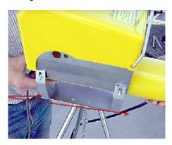
2. Route Propane Hose through center of Tripod Platform.
