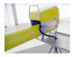
4. Extend Inner Megaphone by loosening the nut and pulling the barrel out.
