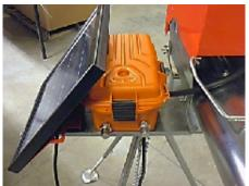
2. Attach the negative wires from Scare Cannon and Solar Panel to the negative (black) alligator clip leads.
