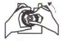
Never hold the Milled Nut (#320 J) while holding the Drive Unit (#320 A). This could cause damage to the Drive Unit.
